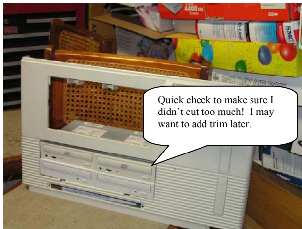
Figure 7 First test fit for side-by-side optical drives – need ¼” more room
