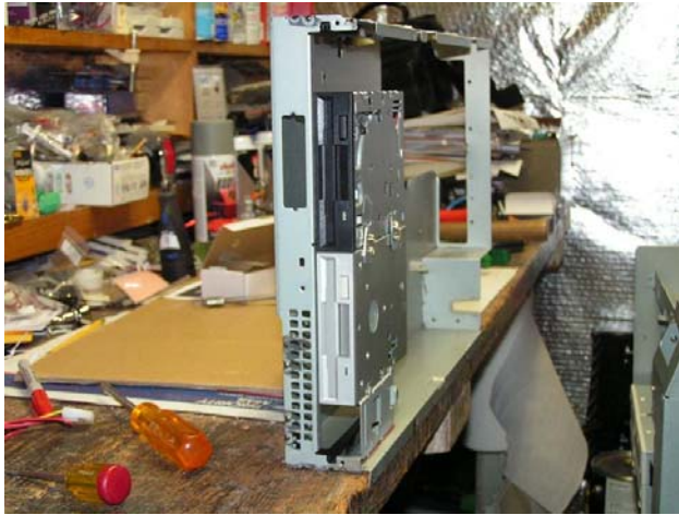
Figure 14 Pair of floppy drives mounted in rear, to internal side panel
