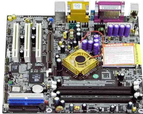
Chaintech 7NIL1-Summit Nforce2 Ultra 400 micro-ATX motherboard (x2)
