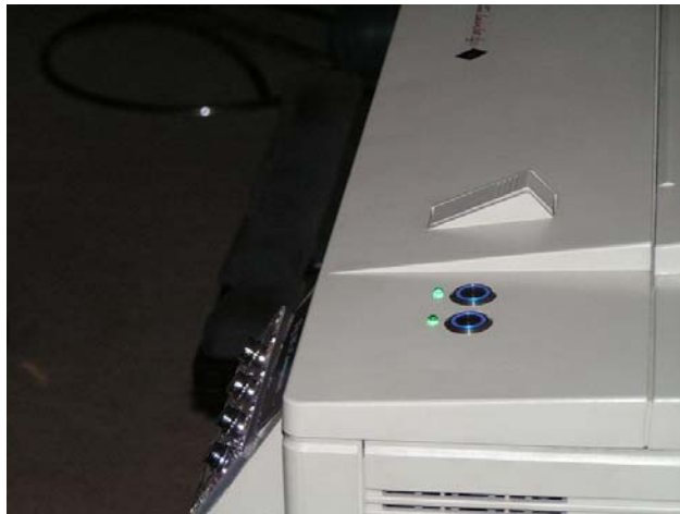
Figure 25 Final install of the power switches and hard drive LEDs
