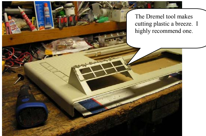
Figure 17 Cutting out the stock LCD / switch panel assembly panel
