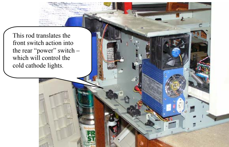
Figure 11 Raidmax "500 W" power supply for secondary motherboard
